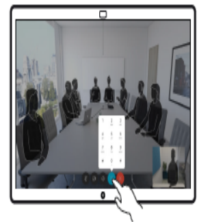
In a call tap the screen to produce the buttons as shown. Then tap the blue button to open the numerical keypad.
